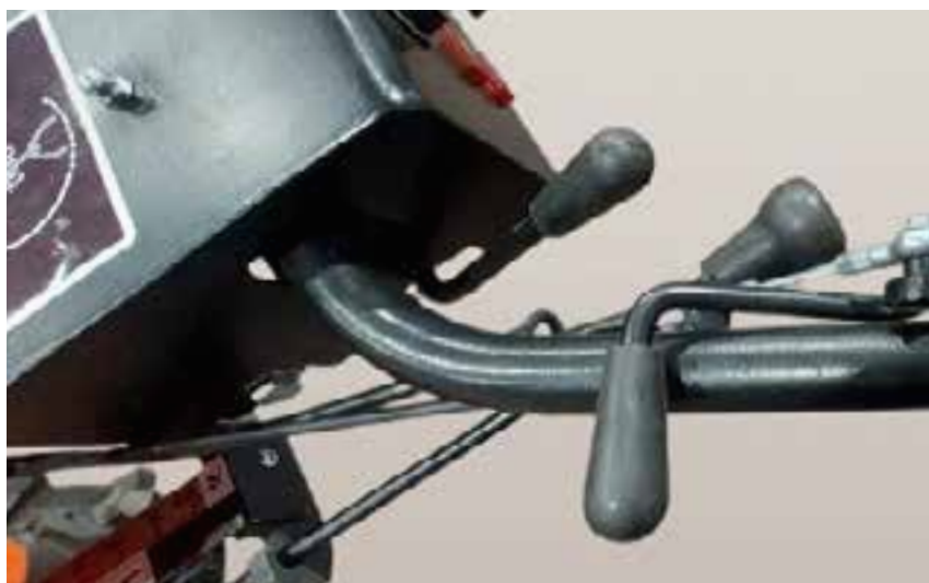
Picture 12 - Lever for moviment handlebars vertically
