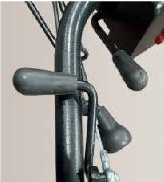
Picture 10 - Lever for moving handlebars horizontally
